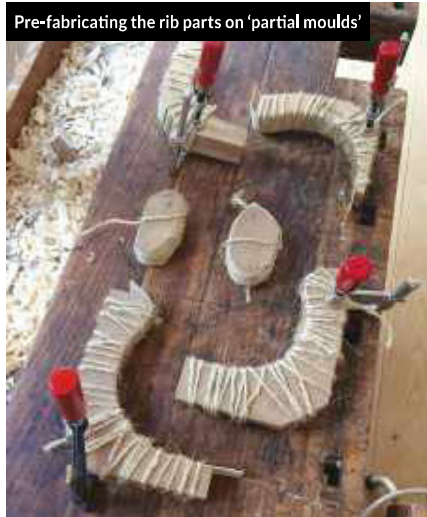
Gluing the pre-formed rib parts on to the internal blocks
