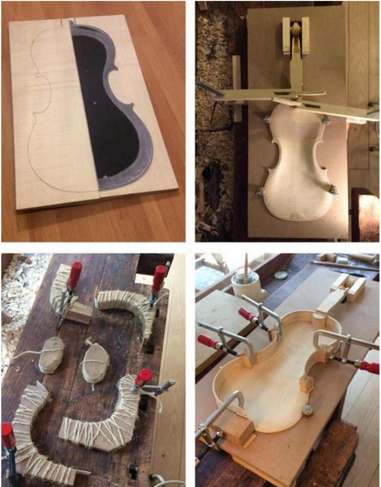
Figure 6.3. Several representative steps in the 2017 construction process of a violin replica after Bousu. Top row, left to right: (a) marking the back plate contour (template produced from CT data), (b) gluing the neck to the back plate using an alignment table. Bottom row, left to right: (c) making the rib parts on partial moulds, clamping is done by rope, (d) gluing the rib parts, including their linings, to the internal blocks.
