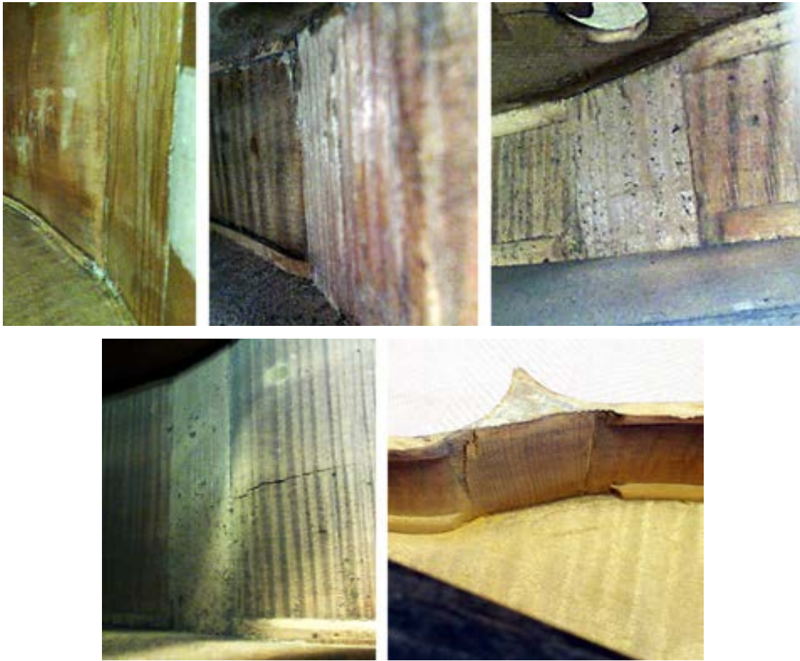
Figure 4.39. Examples of corner blocks in five instruments by Boussu. Top row, left to right: (a) corner block in a cello from 1749 (database code BJB4901vc), (b) corner block in a violin from June 1751 (database code BJB5103vn), (c) corner block in a violin from June 1753 (MIM inv. no. 2784; database code BJB5302vn). Bottom row, left to right: (d) corner block in a cello from 1757 (MIM inv. no. 1372; database code BJB5701vc), (e) corner block in an undated violin (database code BJBnd01vn).
