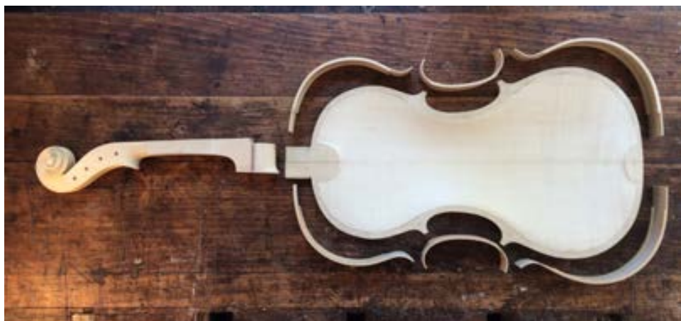
Figure 6.4. A modular system: several prepared violin parts ready to be assembled. Linings are pre-installed on the rib parts, thereby preserving the bent shape of the ribs.
