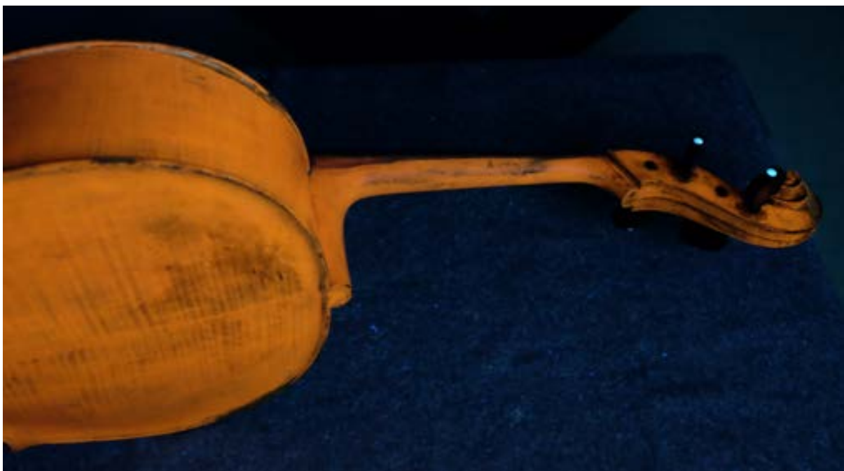
Figure 4.67. UV-induced fluorescence of the varnish on a cello by Boussu from 1757 (MIM inv. no. 1372; database code BJB5701vc).
