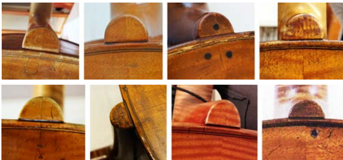
Figure 4.63. Examples of the channel found below the button of the back plate. Top row, left to right: (a) button channel on a cello from 1749 (database code BJB4901vc), (b) button channel on a violin from 1750 (MIM inv. no. 2781; database code BJB5001vn), (c) button channel on a violin from 1751 (MIM inv. no. 2785; database code BJB5101vn), (d) button channel on a violin from June 1751 (database code BJB5103vn). Bottom row, left to right: (e) button channel on a cello from 1751 (database code BJB5104vc), (f) button channel on a cello from January 1752 (MIM inv. no. 2863; database code BJB5201vc), (g) button channel on a cello from June 1752 (database code BJB5202vc), (h) button channel on a violin from August 1752 (database code BJB5203vn).
