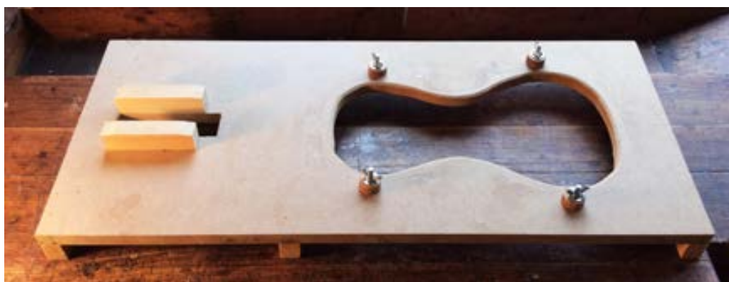
Figure 5.4. Alignment table as made and used by the author for making three violin replicas.
