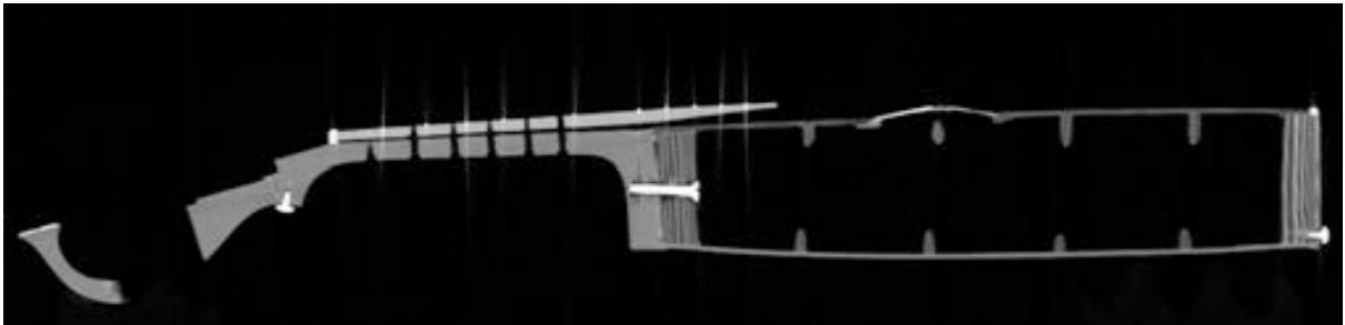
Figure 4.81. Cittern by Boussu (database code BJB7101ci), sagittal plane reconstruction of CT data: longitudinal cross section along centreline.
