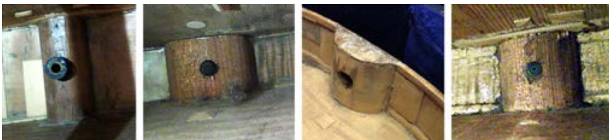
Figure 4.42. Endoscopic captures of the lower block area of four instruments by Boussu. Left to right: (a) lower block in a cello from 1749 (database code BJB4901vc), (b) lower block in violin from June 1751 (database code BJB5103vn), (c) lower block in an undated violin (database code BJBnd01vn), (d) lower block in an undated viola (database code BJBnd16va).
