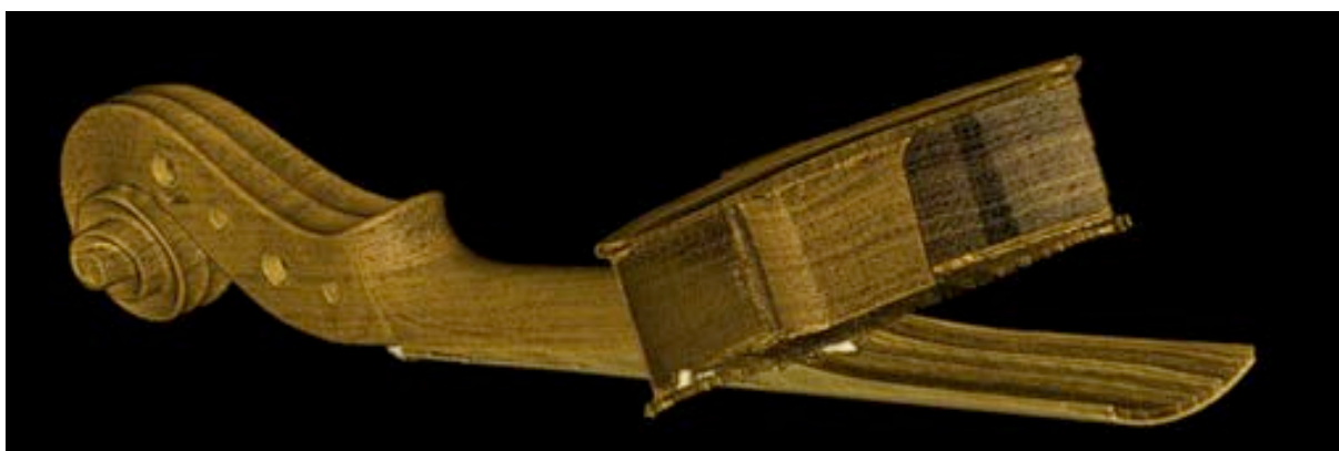
Figure 4.55. 3D volume render of CT scan data for a violin by Boussu dated 1750 (MIM inv. no. 2781; database code BJB5001vn), detail of the neck and fingerboard. Note: part of the sound box has been erased from the reconstruction.
