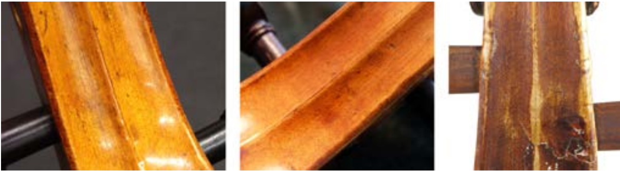
Figure 4.14. Scribe lines on the spine of the pegbox and scroll. Left to right: (a) scribe line on the central spine of the pegbox on a violin from June 1751 (database code BJB5103vn), (b) scribe line on the central spine of the pegbox on a viola from 1759 (database code BJB5901va), (c) scribe line on the central spine of the scroll on a violin from 1765 (database code BJB6501vn).
