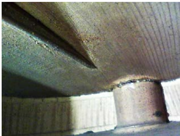
Figure 4.45. Endoscopic capture of the bass bar area of a violin by Boussu from June 1753 (MIM inv. no. 2784; database code BJB5302vn).
