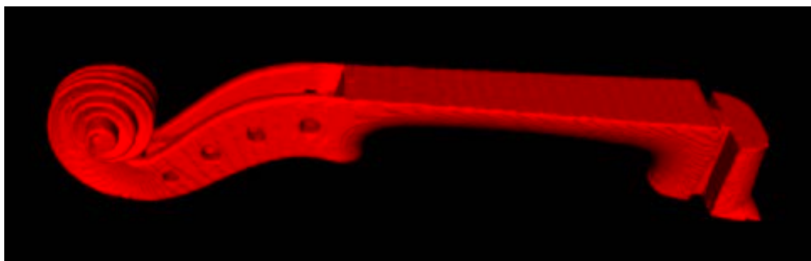
Figure 6.14. Example of CT data segmentation: a reconstruction of the neck/upper block/scroll combination of a violin by Boussu (MIM inv. no. 2781; database code BJB5001vn).
