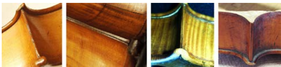
Figure 4.33. Examples of the connection of two rib parts at a corner of the garland. Left to right: (a) rib corner in a violin from 1750 (MIM inv. no. 2781; database code BJB5001vn), (b) rib corner in a cello from 1757 (MIM inv. no. 1372; database code BJB5701vc), (c) rib corner in a violin from 1759 (database code BJB5903vn), (d) rib corner in an undated violin (database code BJBnd01vn).
