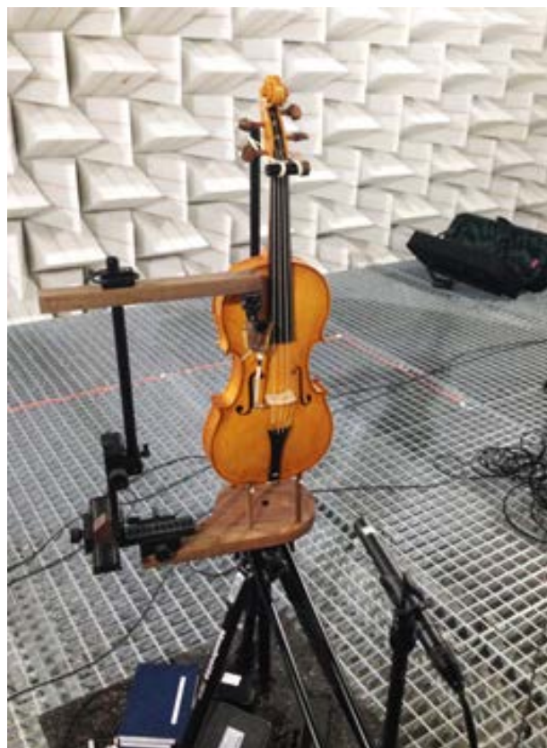
Figure 6.15. Measurement set-up for acoustic radiation measurements on the replica violins, at the anechoic chamber of UPMC/Institut Jean Le Rond d'Alembert.
