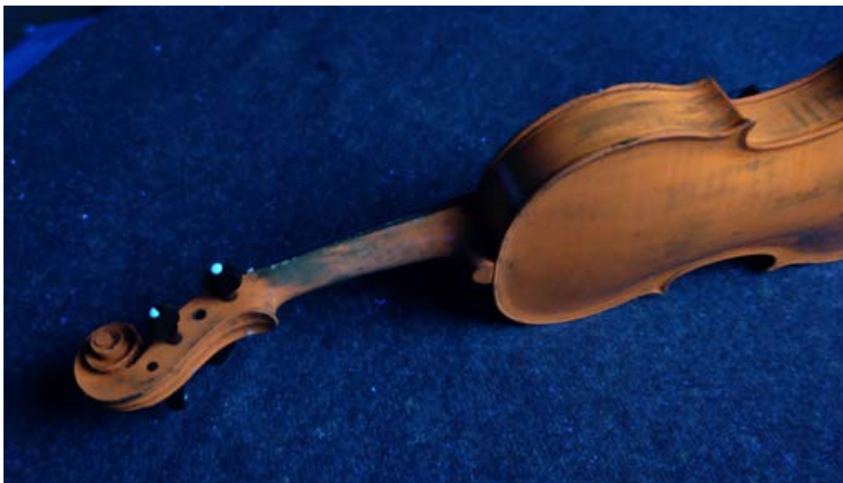
Figure 4.66. UV-induced fluorescence of the varnish on a violin by Boussu from 1750 (MIM inv. no. 2781; database code BJB5001vn).
