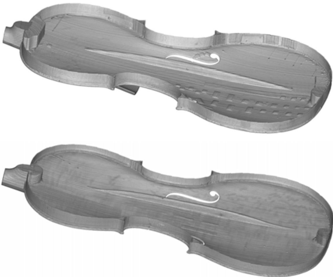
Figure 4.48. Inside views of the top plate of two cellos by Boussu. Top to bottom: (a) inside of top plate of a cello from January 1752 (MIM inv. no. 2863; database code BJB5201vc), (b) inside of top plate of a cello from 1757 (MIM inv. no. 1372; database code BJB5701vc). Images obtained by 3D volume rendering of CT scan data, with greyscale values inverted.
