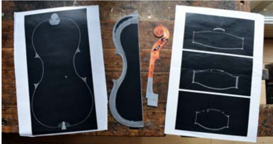
Figure 6.1. Examples of scale 1:1 construction plans and templates, based on the CT scan data of the Boussu violin with MIM inv. no. 2781 (database code BJB5001vn).
