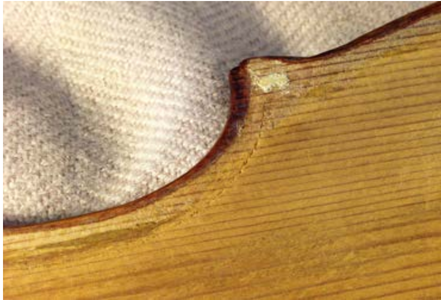
Figure 4.16. Scribe line at the inside of the top plate of an undated violin (database code BJBnd01vn).
