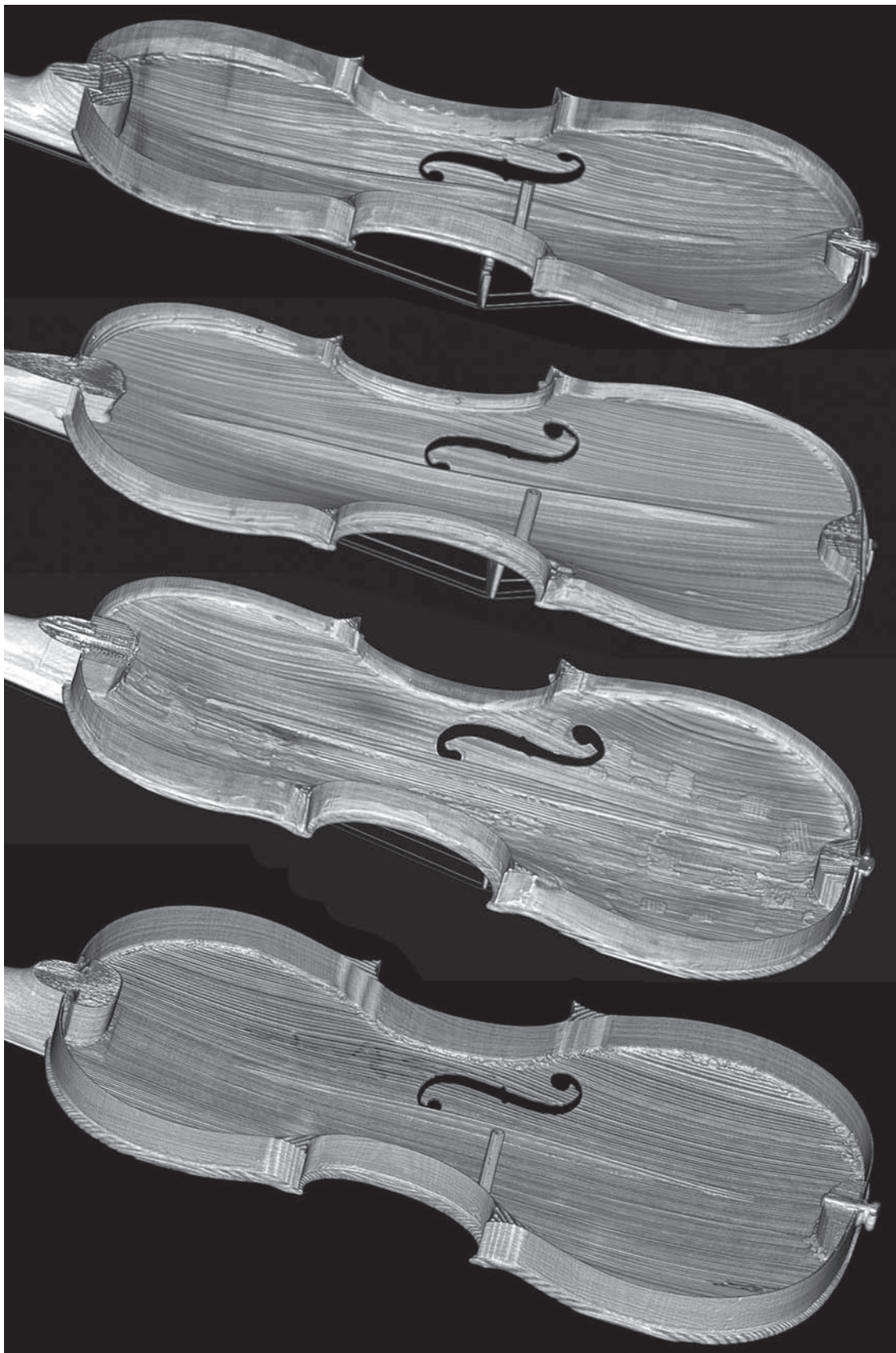
Figure 21. Inside views of the top plate in the four instruments: (a) violin by Jan de Maseneer, MIM inv. no. 2786; (b) violin by Gaspar Borbon, MIM inv. no. 2774; (c) violin by Egidius Snoeck, MIM inv. no. 2779; (d) violin by Benoit-Joseph Boussu, MIM inv. no. 2781. Images obtained from 3D volume rendering of CT-scan data.
