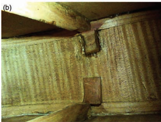
10 Cittern branded 'BOUSSU', endoscopic captures of interior: (a) upper block area; (b) braces on top and back plates
